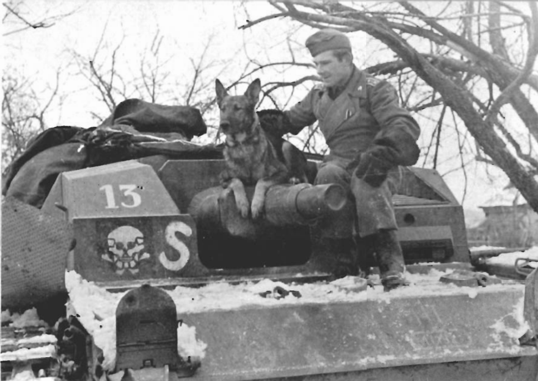
A useful high view of an ausf B, showing the stowage and rear hull details; note the railing that supports the spare track. [National Archives]
