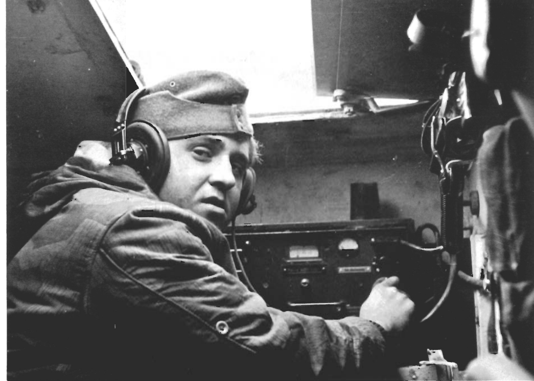
StuG III ausf G's, radios were carried only on the left below the cupola and were intended for the vehicle commander. Command and observation vehicles had extra radios on the right side wall, as shown here.
