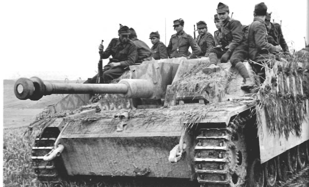
Two views of a slightly later production StuG III ausf G. The nose armor is 80 mm base, and the raked zimmerit pattern is used. The camouflage paint was applied with a sponge. Hungarian infantry ride on these German vehicles during the campaign in southern Russia. Note the "C" tow hooks hung in the front two shackle holes.
