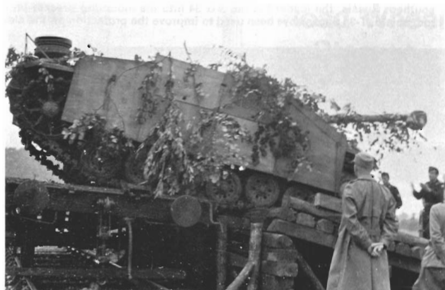
An ausf G being driven off a flatcar, showing a common way of attaching foliage to a vehicle. Merely hooking the inverted branches over the upper edge of the skirting was sufficient to hold them in place—until the vehicle went through heavy brush or undergrowth. [Bundesarchiv]
