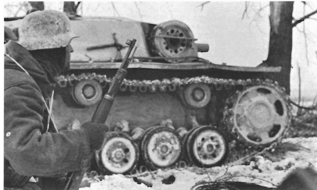
This snow-camouflaged ausf B shows the altered front roller and later cast dished drive sprocket introduced with the 40 cm wide track.
