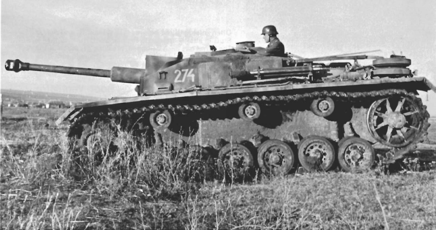
Another ausf F retaining the ausf E superstructure front. Again, the L/48 has been refitted, and some paint has been burned off the muzzle brake. Another type of winter clothing is shown here. [Bundesarchiv]
