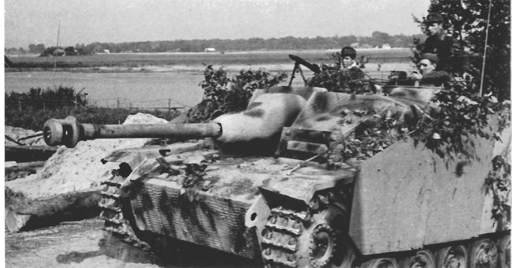
Another later ausf G in France. It is dark yellow with dark green patches. As was rather common with StuG III's, the gun barrel is darker than the rest of the vehicle, perhaps as a result of heat from extended firing.
