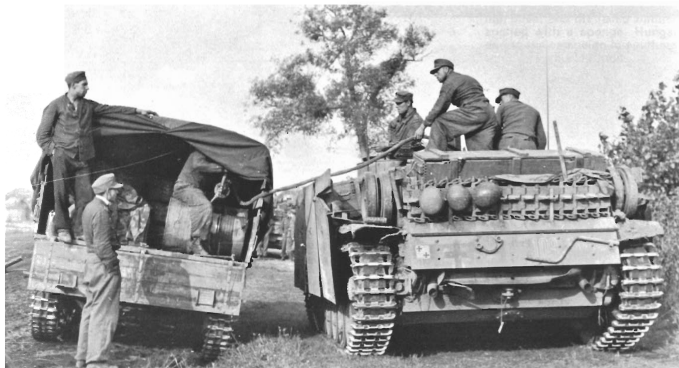
Two StuG III ausf G's in Italy, 1944. Both vehicles carry large fuel drums and the "waffle plate" zimmerit coating. The men on the vehicles are infantry and StuG III crewmen.
