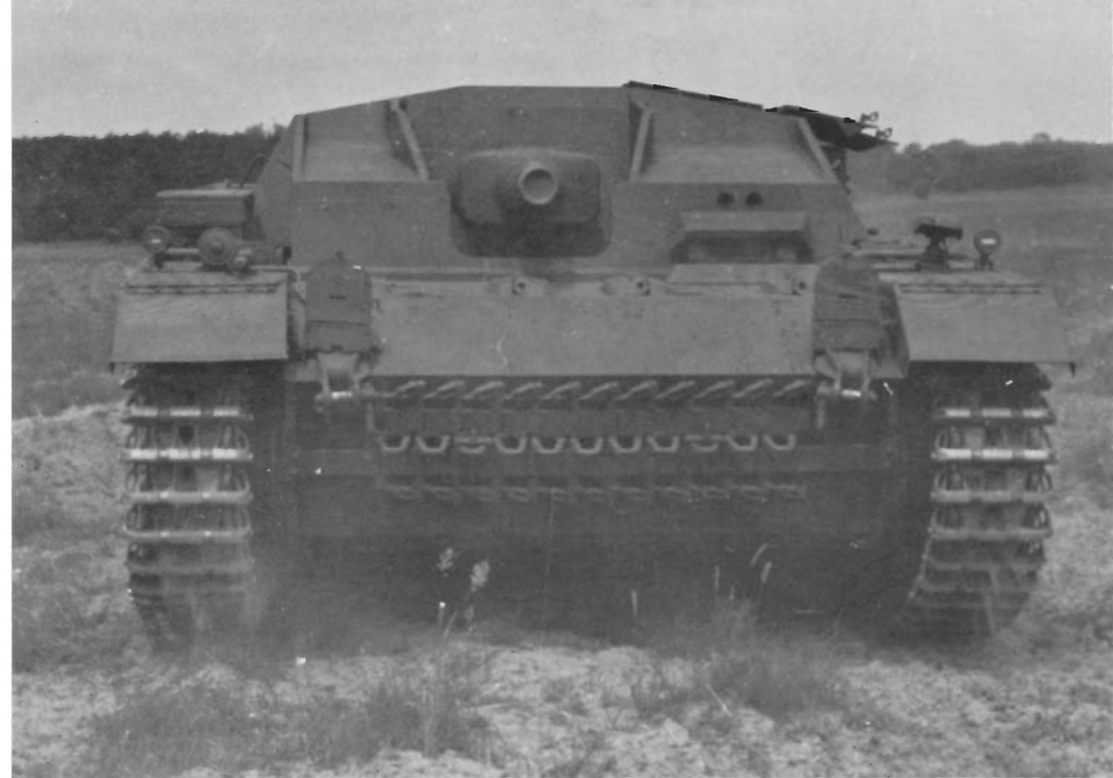
This front view of a new StuG III ausf C shows the redesigned superstructure which eliminated the front aperture for the gunner's sight; this was now mounted in the roof. The two holes over the driver's visor are for the driver's binocular vision device ["fahrerfernrohr"].
