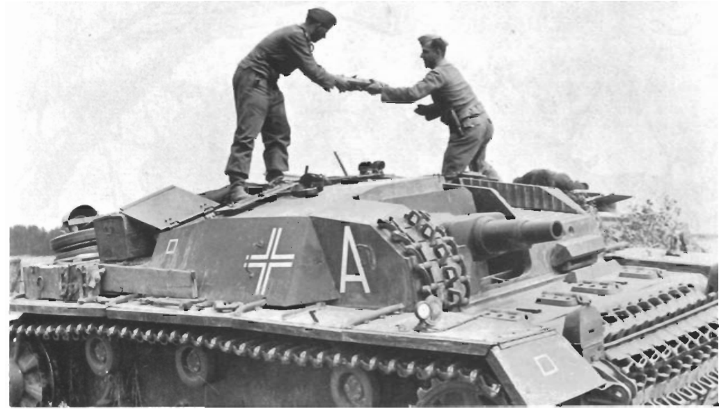
Two crewmen load ammunition into this StuG III ausf B. The relocated front return roller can be seen. Note the extra track up front, and the original built up rear idler. The extra tracks not only provided some extra protection, but could also be used in field repairs for the vehicle's tracks. [Bundesarchiv]
