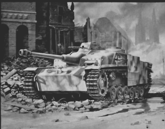
Late StuG III ausf G of the Panzer Lehr Division, 1945. This vehicle, camouflaged in Dark Yellow and Green Camouflage, has the rare late addition of concrete re-inforcement to the superstructure.
