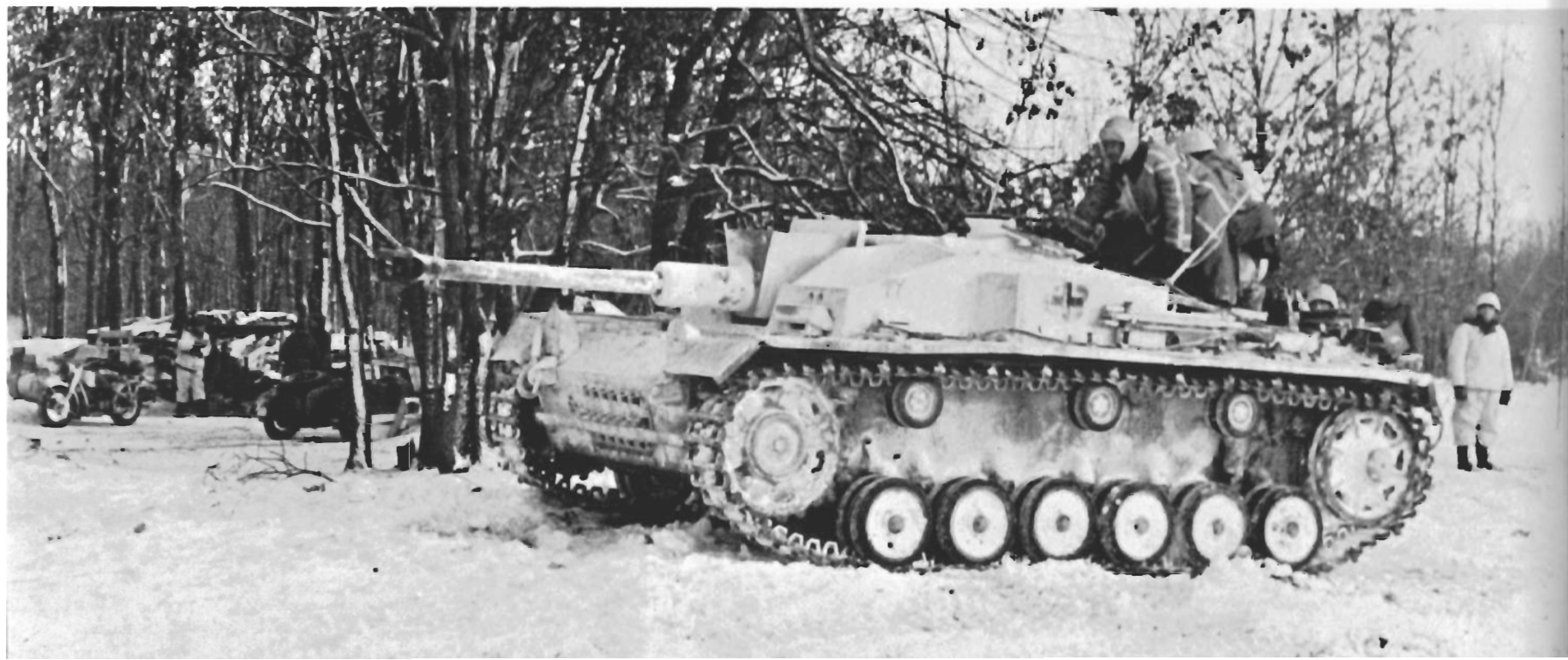
Another ausf F retaining the ausf E superstructure front. Again, the L/48 has been refitted, and some paint has been burned off the muzzle brake. Another type of winter clothing is shown here. [Bundesarchiv]
