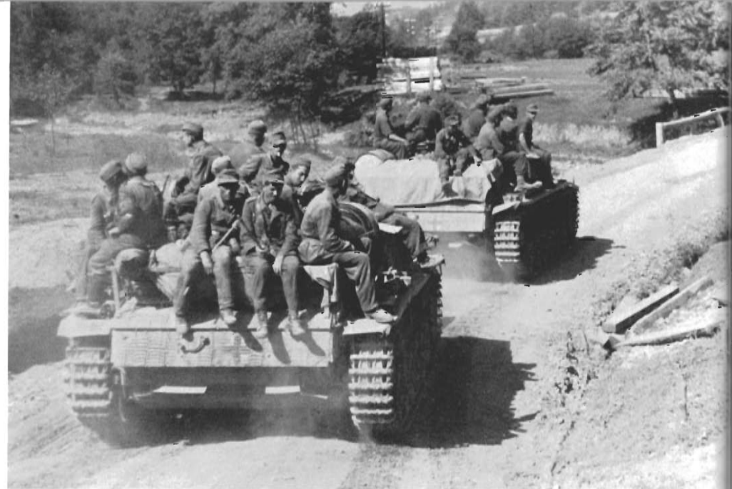
Two StuG III ausf G's in Italy, 1944. Both vehicles carry large fuel drums and the "waffle plate" zimmerit coating. The men on the vehicles are infantry and StuG III crewmen.
